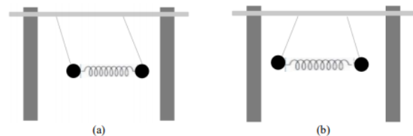
Figure 1. Spring coupled pendulum oscillatory with (a) in-phase and (b) out-of-phase motions.
