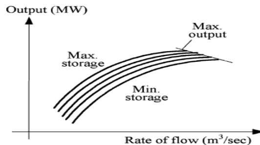
Figure 2. Input-Output feature by a typical pumped-storage plant in power generation mode
