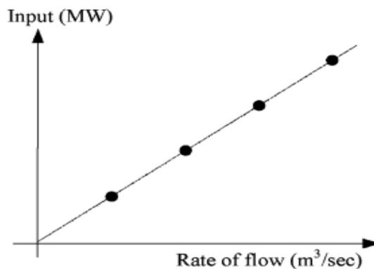
Figure 3. Input-output characteristic of a typical storage pump unit in pumping mode
