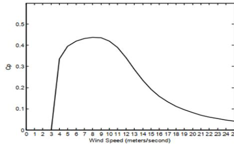
Figure 4. Efficiency of the turbine vs. instantaneous wind speed
