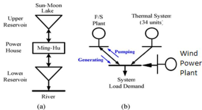
Figure 8. Real plant system. (a) Hydraulic diagram (b) electric diagram
