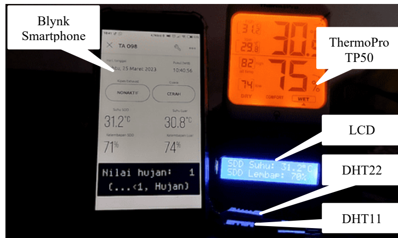
Figure 7. Sensor calibration process with ThermoPro. Information for figure, Nilai hujan is a description of the value of rain, hujan is a description of rain, suhu is a description of temperature, lembap is a description of humidity
