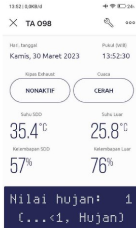
Figure 10. Blynk view when the weather is clear. Information for figure, Kamis is a description of Thursday, Waktu is a description of the time display in the form of hours, Nilai hujan is a description of the value of rain, hujan is a description of rain, suhu is a description of temperature, kelembapan is a description of humidity, cuaca is a description of weather, cerah is a description of sunny
