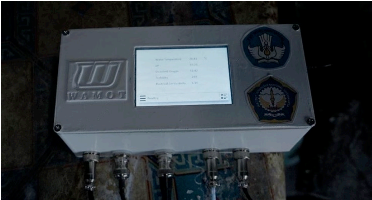
Figure 9. Integrated the liquid waste monitoring system based on internet of things tools
