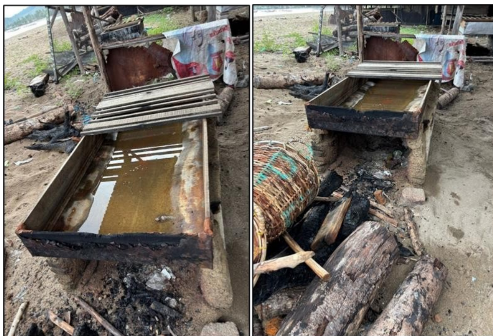
Figure 4. Traditional mixed-material boiling equipment and firewood-based heating were used before the technology transfer
