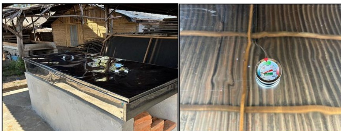
Figure 5. Food-grade stainless-steel boiling vessel with gas-based heating and a temperature gauge for controlled anchovy boiling
