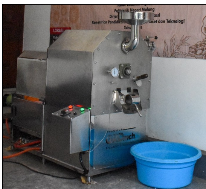
Figure 1. Controlled coffee bean rotary dryer machine with a capacity of 30 kg.
