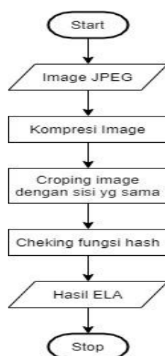
Fig. 1 Error Level Analysis Method Flow
