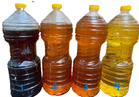
Fig 4. Unprocessed (1) Processed used cooking oil(2 &3) and fresh unused cooking oil (4)
