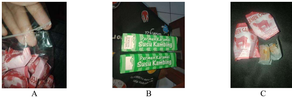
Figure 1. Types of defects that occur in goat's milk caramel candy products; (A) damaged packaging, (B) no expiration label, and (C) torn packaging.
