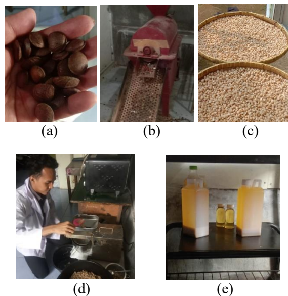
Figure 1. Stages of sachai inchi oil extraction: (a) sachai inchi seeds; (b) seed shelling equipment; (c) seed drying process; (d) seed pressing to obtain oil; (e) sachai inchi oil obtained.
