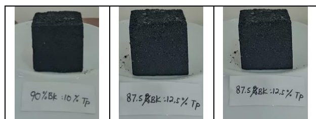
Figure 2. Biobriquettes made from ketapang fruit with variations in the percentage of tapioca paste
