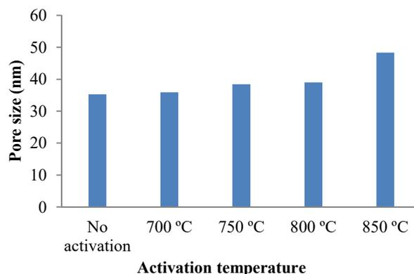
**Figure 3.** The effect of the activation temperature on the activated charcoal oil palm pore
