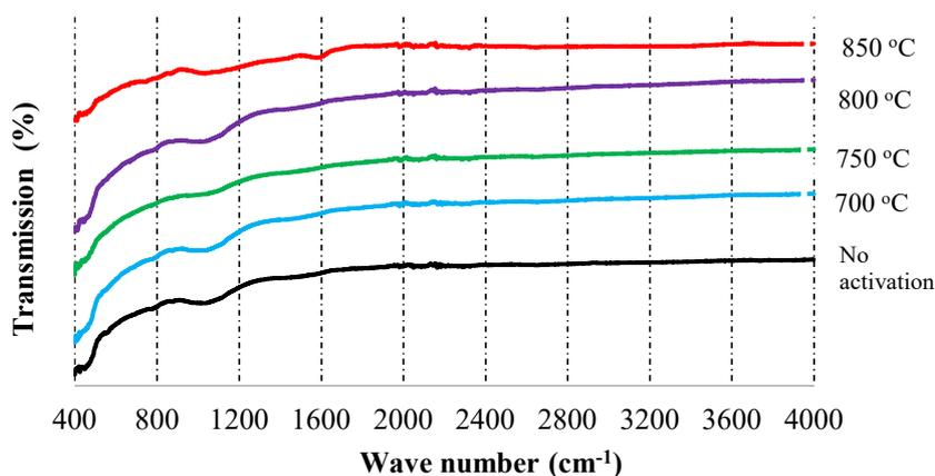
**Figure 4.** IR spectrum of activated charcoal from palm shells with activation temperature variations
