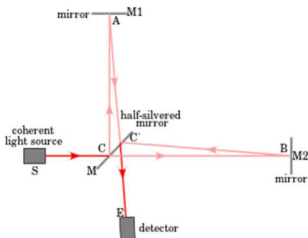
Figure 1. Michelson interferometer design[19]
