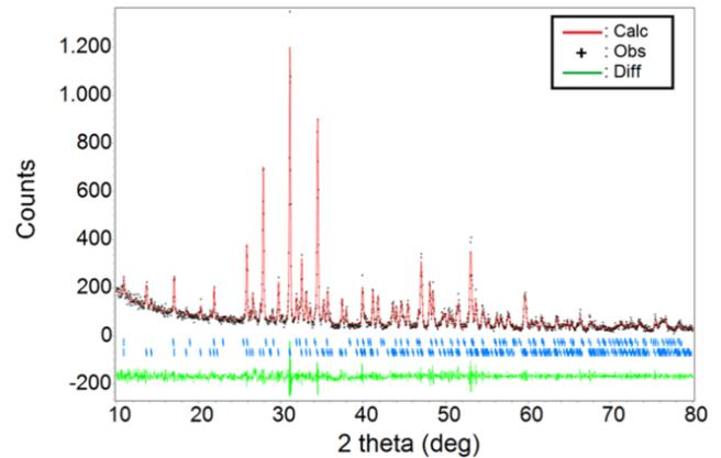
**Figure 3.** XRD pattern of calcium phosphate synthesized from cockle shell waste. The + symbol indicates the experimental data (obs), and a solid line indicates the calculation (calc) of the refinement. The lower trace is the difference between experiment and calculation (diff). The vertical lines mark the position of the calculated Bragg peaks for an HA and  $\beta$ -TCP, respectively.
