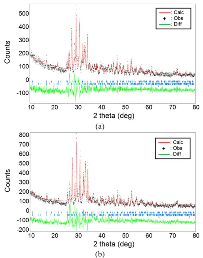
**Figure 7.** XRD pattern of calcium phosphate loaded by silver nanoparticles: (a) TCP3/Ag and (b) TCP5/Ag. The + symbol indicates the experimental data (obs), and a solid line indicates the calculation (calc) of the refinement. The lower trace is the difference between experiment and calculation (diff). The vertical lines mark the position of the calculated Bragg peaks for an HA,  $\beta$ -TCP, and silver nanoparticles, respectively
