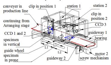
Figure 5. Inspection system with machine vision
