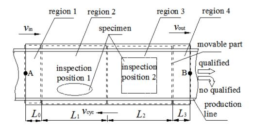
Figure 3. The general layout of the inspection system
