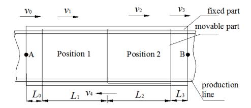
Figure 7. Moving cycle of the inspection system
