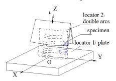
Figure 8. Complete position of the specimen
