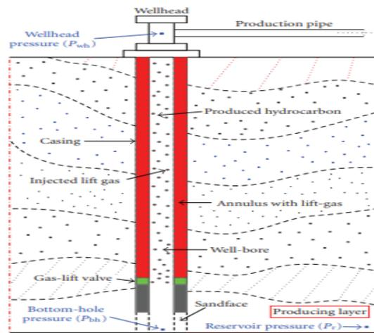
Figure 1. Gas Lift Well Schematic (Rashid et al., 2012)
