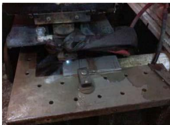
Figure 3. Vickers hardness specimen preparation by WEDM
