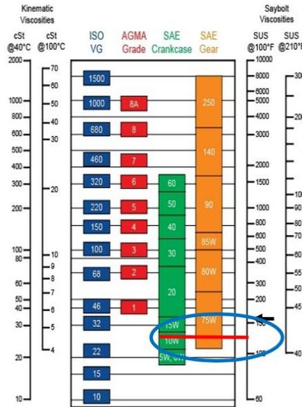
Figure 14. Lubricating oil selection chart based on viscosity
