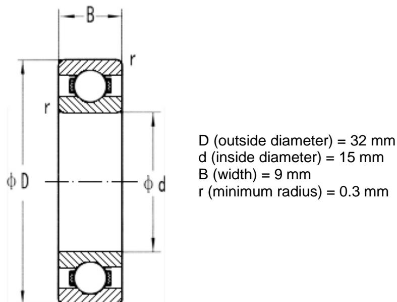
Figure 11. Bearing dimensions
