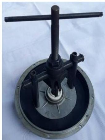
Figure 8. Removal of ceramic bearings
