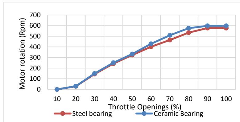
(b) Motor rotation vs. Throttle openings
