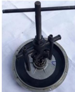
Figure 5. Removing factory default bearing.
