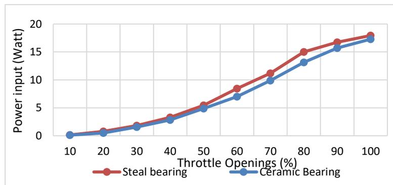
(a) Input power vs. Throttle openings
