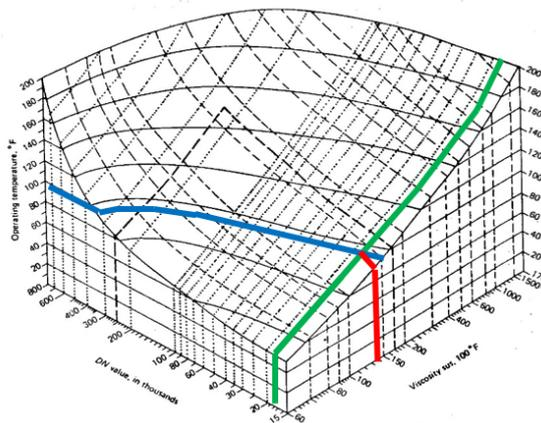
Figure 13. Lubricating oil selection chart based on viscosity
