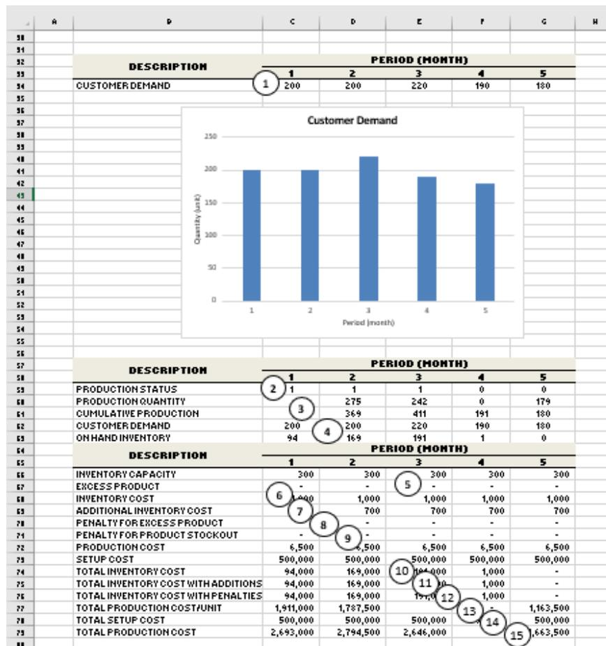
Figure 2. The lot sizing model using spreadsheet in Microsoft Excel software
