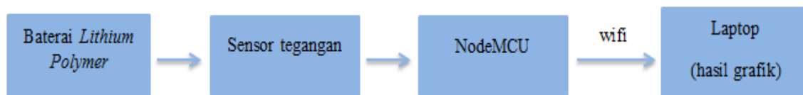
Gambar 1. Diagram blok perancangan hardware
