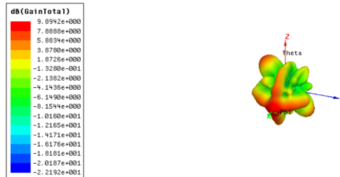
Figure 20. Gain of the cross-configured 4-port MIMO antenna at 10.7 GHz
