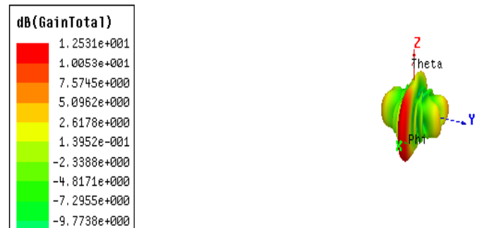
Figure 22. Gain of the cross-configured 1 \times 4 MIMO antenna at 6.7 GHz
