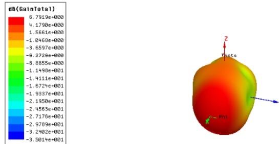
Figure 11. 3D gain plot of the reference antenna at 8.7 GHz
