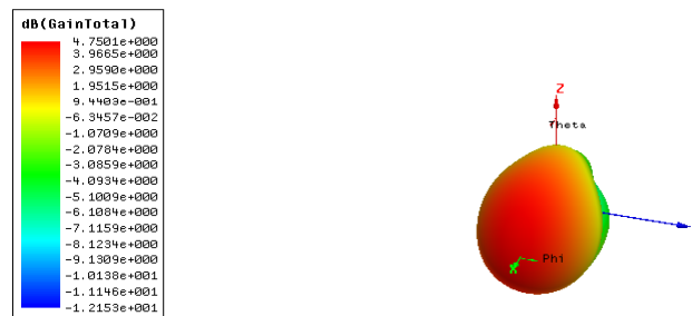
Figure 10. Gain results for the reference antenna at f_r = 6.7 GHz
