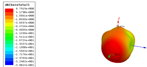
Figure 14. Bow-tie-inspired antenna with directors and lens-shaped modification gain at f_r = 8.7 GHz
