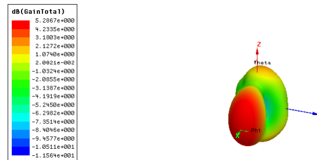
Figure 11. Gain results for the reference antenna at f_r = 8.7 GHz
