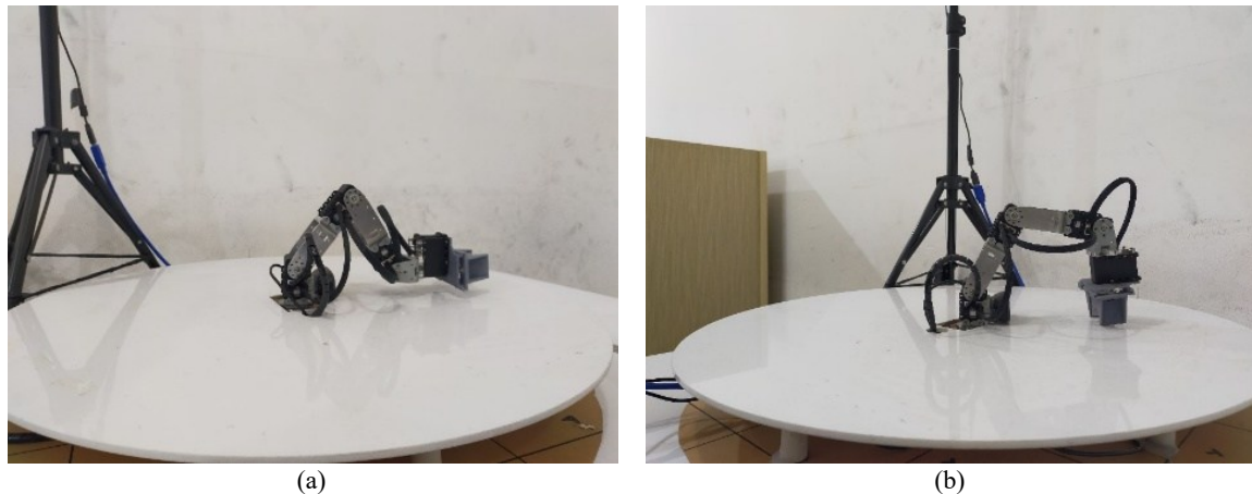
Figure 11. Experimental setup for inverse-kinematics evaluation: (a) Frontal retrieval configuration; (b) Top-down retrieval configuration
