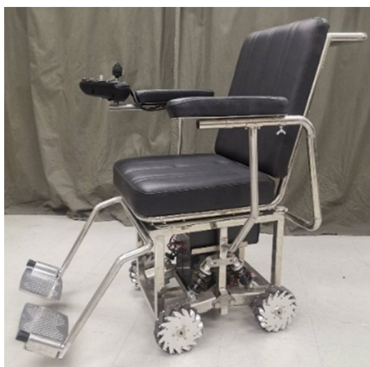
Figure 2. Electric Cart Control System with Mecanum Wheels
