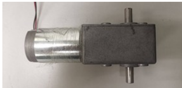
Figure 3. DC Motor Used in the Mecanum Wheel System
